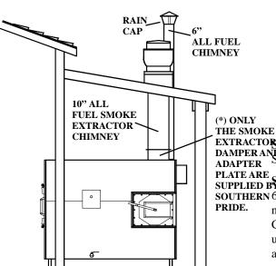
**NOTE 1.** When installing an Oven through a wall constructed of combustible material, use the **Southern Pride Insulation Kit** between the oven and the wall.
